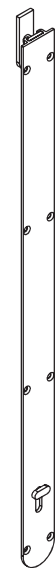
No. 456LN LONG NECKED FLUSH BOLT 600mm x 41mm with 11mm mortice, 20mm throw and 9mm offset
