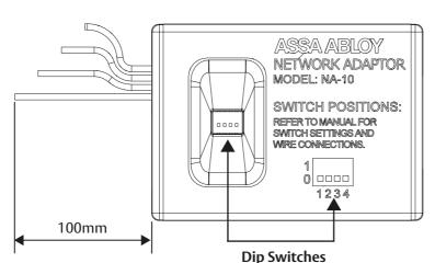
Ensure that dip switches are all in the down or off position as shown. This is the default position.
