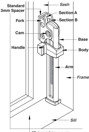
**NB:** For installation on awning windows, the safety stay should be installed as close to the bottom sill as possible to restrict the window opening width.
