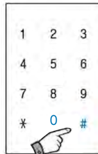
3. Press 0 + # keys, all data will be deleted
