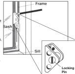
· Locking pin on sash plate must be facing away from window frame as shown on diagram.
